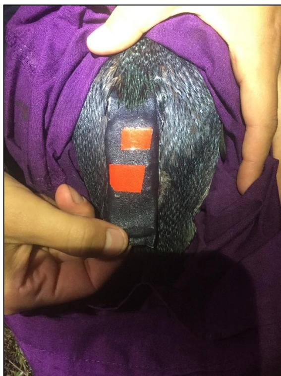
Figure 1. An I-GotU GT120 GPS logger attached to the lower back feathers of a little penguin using waterproof TESA tape and superglue
