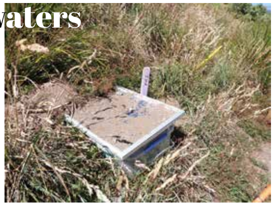
▲ PIT reader with solar panel covered by shearwater-excavated soil.
