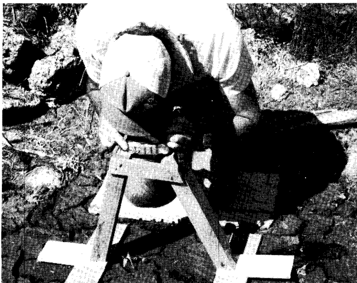
FIGURE 1 — For long film exposure a special stand was used to position the lens 450 mm above the ground surface.
