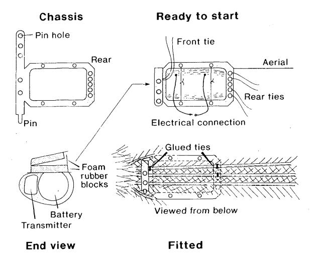
FIGURE 2 - Method of construction and attachment of the transmitter package used on Chatham Island Taiko in 1987
