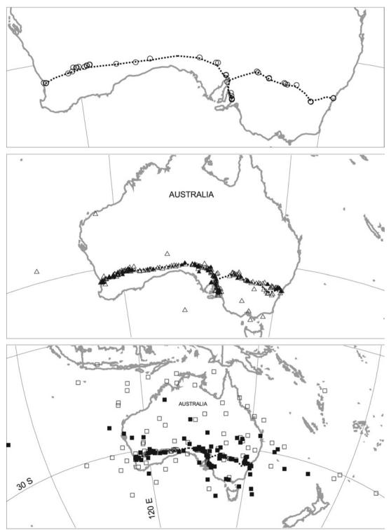
**Fig. 3** Comparative 'location' distributions for PTT #899 when carried by a transcontinental train on multiple trips across southern Australia between 12 Aug and 9 Dec 1999.  $\circ$ , LC =3, 2, 1;  $\triangle$ , LC =0;  $\blacktriangle$ , LC =A;  $\blacksquare$ , LC =B;  $\Box$ , LC =Z. Broken line represents actual route train.
