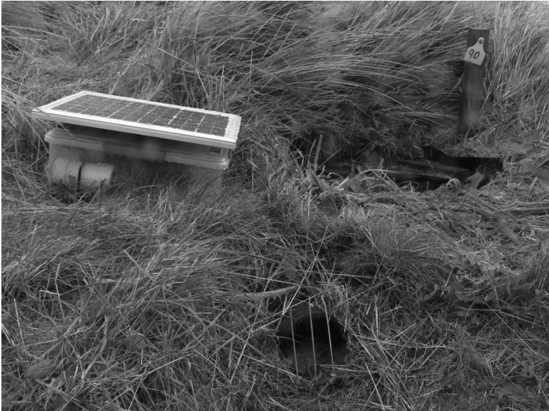
Fig. 2. Nestbox 90 with pins at the tunnel entrance and the PIT reader assembly.
