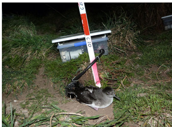
Fig. 3. Hutton's shearwater at the entrance to burrow C20 at the Kōwhai River colony with the antenna coil in place and attached to the reader assembly. (Photo L. Rowe)
