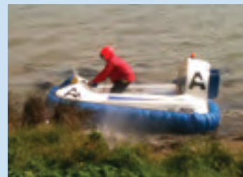
< HOVPOD. THIS PIECE OF EQUIPMENT IS USED TO SCARE OFF BLACK SWANS THAT ARE CONGREGATING IN THE BAY WEST OF THE AIRPORT AND 200 M NORTH OF THE ACTIVE RUNWAY. OUR AIM IS TO USE THIS DAILY SO THAT THE SWANS DO NOT ASSOCIATE THE BAY AS A SAFE HAVEN.
