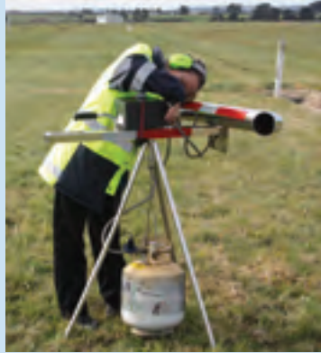
GAS CANNON. THIS IS USED ON GRASS AREAS TO FRIGHTEN BIRDS, AS IT LETS OF CONSECUTIVE LOAD BANGS. IT CAN BE SET ON A TIMER OR USED BY REMOTE CONTROL. IT IS VERY EFFECTIVE FOR THE CONTROL OF SEED EATING BIRDS (FINCHES, YELLOWHAMMERS AND SKYLARKS IN SUMMER). IT IS ALSO VERY SUCCESSFUL FOR THE CONTROL OF SPUR-WINGED PLOVERS AND HERONS FEEDING ON THE WET GRASS AREAS IN WINTER MONTHS.
