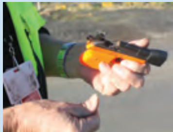
SCREAMER AND BANGER GUN. THIS GUN IS VERY EFFECTIVE TO CONTROL BIRDS IN FLIGHT FROM 0-100 M AWAY. IT CAN BE LOADED WITH A SCREAMER, WHICH SETS OF A LOUD, LONG SCREAM WHEN FIRED. IT CALL ALSO BE LOADED WITH A BANGER, WHICH LETS OFF ONE LOAD BANG WHEN REACHED ITS MAXIMUM DISTANCE. THIS GUN IS PREDOMINANTLY EFFECTIVE FOR SCARING HARRIERS, GULLS AND OTHER BIRDS THAT ARE MOST COMMONLY ENCOUNTERED IN FLIGHT.
