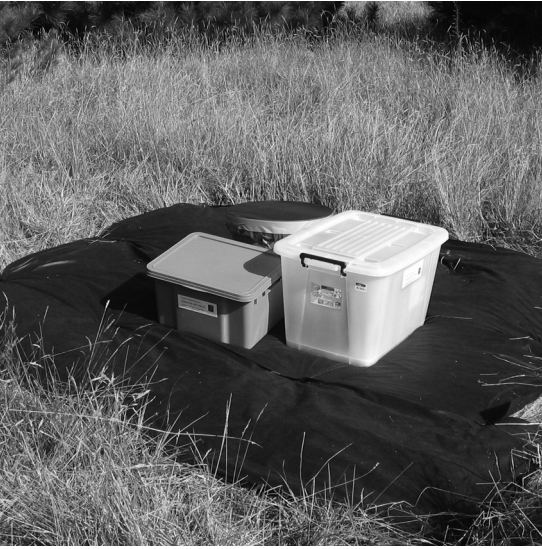
Fig. 1. A bioacoustic unit situated in rank grass. The 2 containers in the foreground house the laptop (left) and batteries (right). The microphone element is housed within the ceramic pot placed behind.
