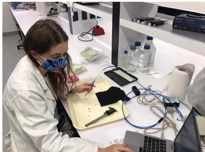
Image 1: Measuring the spectral reflectance plastic colours ingested by seabirds using a spectrophotometer. This will be modelled into a seabird's vision
